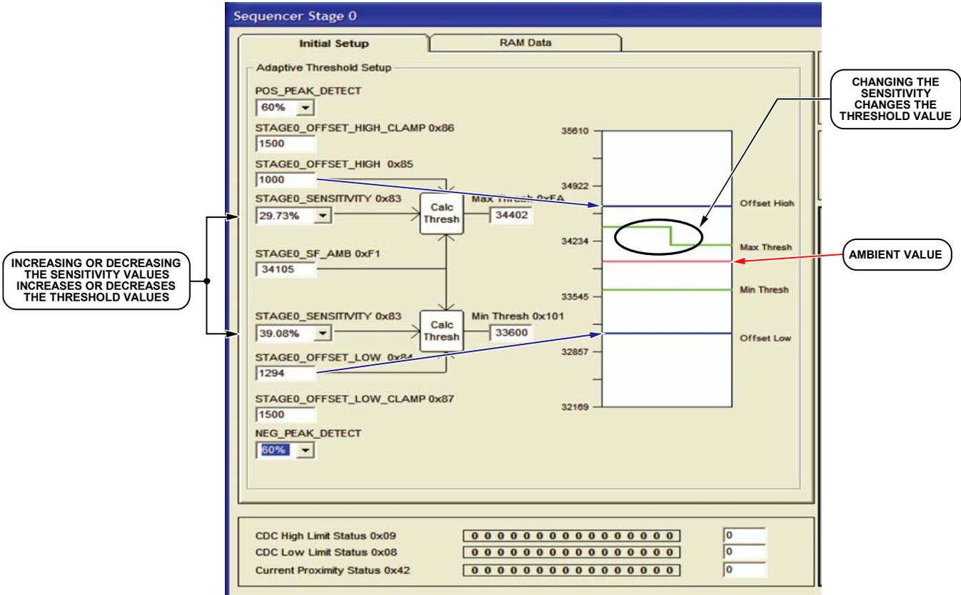
Figure 12. Sequencer Stage 0 Initial Setup Dialog Box
