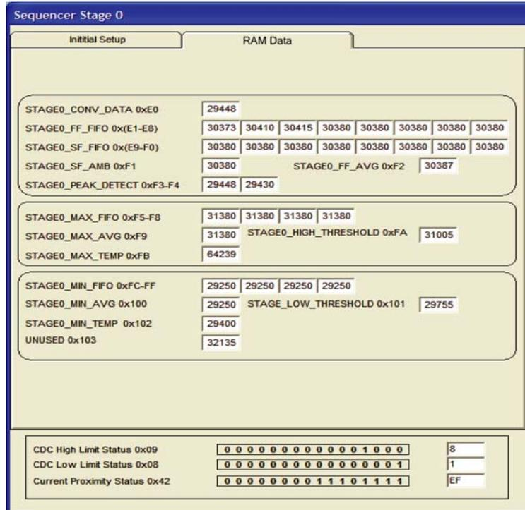
Figure 14. Sequencer Stage 0 RAM Data Dialog Box
