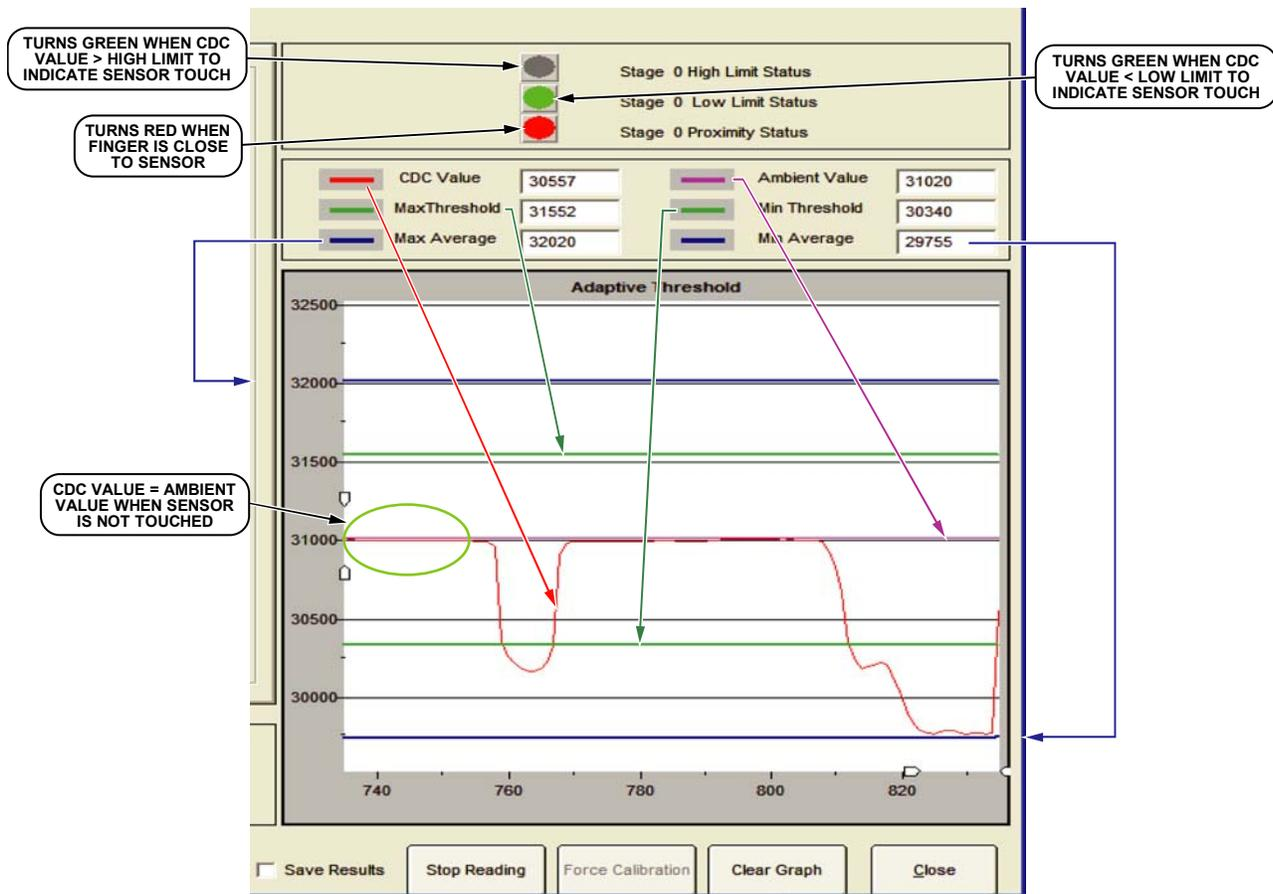
Figure 11. Stage 0 Calibration Engine Dialog Box—Right-Hand Side
