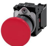
Mushroom pushbutton, 22 mm, round, plastic with metal front ring, red, 40mm, latching, pull-to-unlatch mechanism, with holder, 1 NC, screw terminal, with laser labeling, upper case
