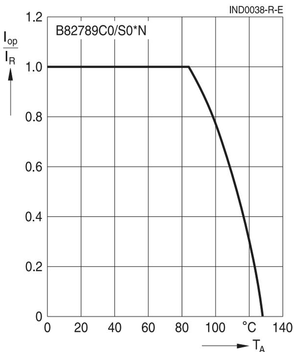
**Current derating  $I_{op}/I_R$  versus ambient temperature** (rated temperature  $T_R = +110 \text{ }^\circ\text{C}$ )
