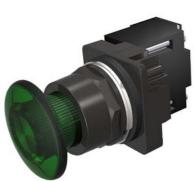
30mm BlackMax, Epoxy Coated Corrosion Resistant Complete Metal Unit Illuminated Push-Pull Operator Full Voltage, 120V AC/DC Incandescent Lamp Mushroom Head Cap Small 1 3/4" (44.5 mm) Plastic, Green 3 Position Momentary UL Listed, CSA Certified NEMA 1,3,3R,4,4X,12,13 & Automotive Standards
