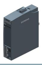
SIMATIC ET 200SP, Digital output module, DQ 16x 24V DC/0.5A STANDARD, Source output (PNP,P-switching) Packing unit: 10 pieces, fits to BU-type A0, Colour Code CC00, substitute value output, module diagnostics for: short-circuit to L+ and ground, wire break, supply voltage
