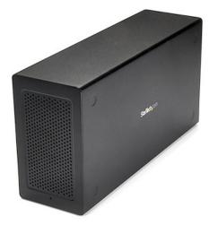
This Thunderbolt3 PCIe expansion chassis lets you add a PCI Express card to your laptop or desktop computer, through an external Thunderbolt 3 connection. The chassis also features a DisplayPort video output, so you can connect an additional monitor to your laptop, and supports Thunderbolt 3 daisy chaining, so you can expand your workstation even further.
