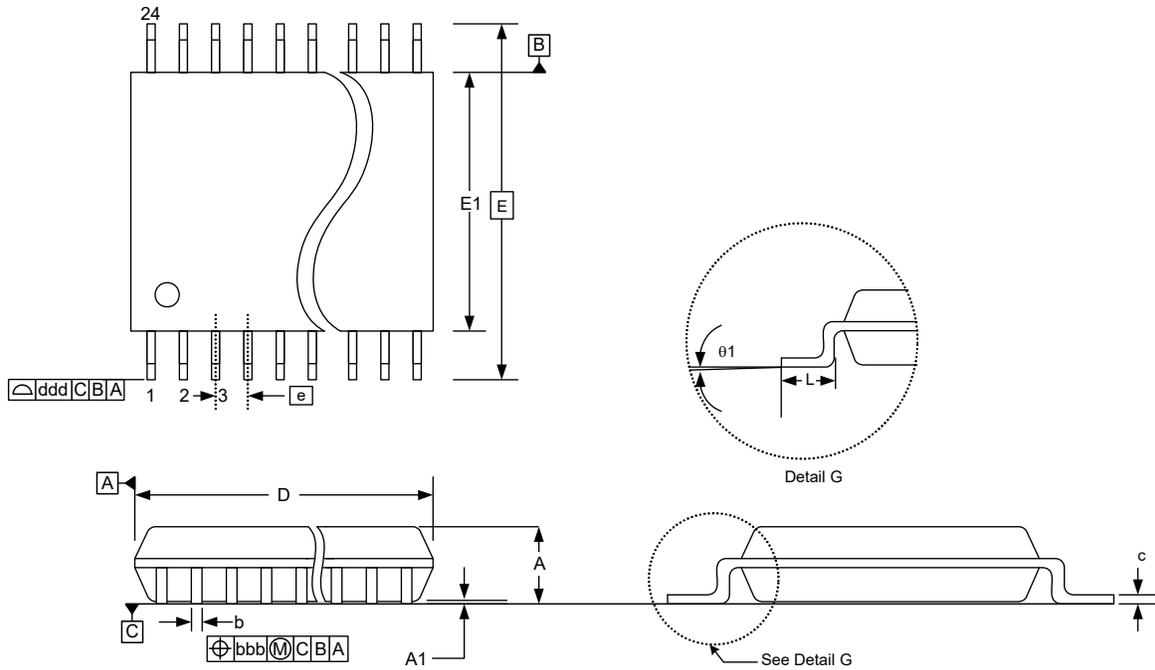
**Figure 19. 24-Pin Thin Shrink Small Outline Package (TSSOP)**
