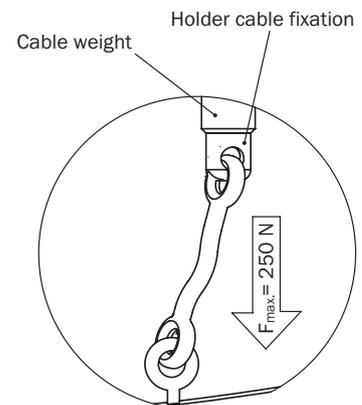
Instruction for installation Installation in a metal immersion tube or metal bypass
