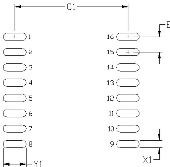
**Figure 7.1. PCB Land Pattern: 16-Pin Wide Body SOIC**
