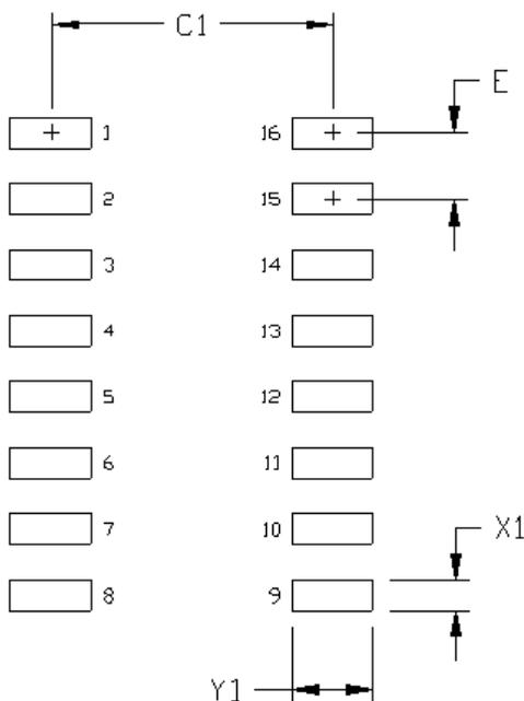
Figure 9.1. PCB Land Pattern: 16-Pin Narrow Body SOIC
