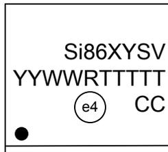
Figure 10.1. 16-Pin Wide Body SOIC Top Marking
