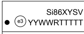
**Figure 11.1. 16-Pin Narrow Body SOIC Top Marking**
