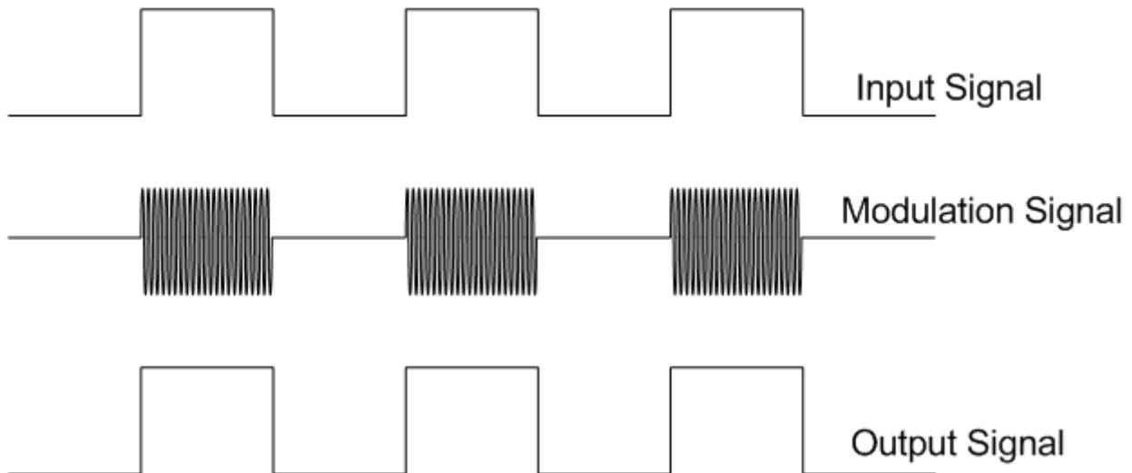
**Figure 2.2. Modulation Scheme**
