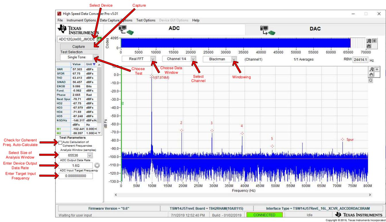
Figure 3-4. High Speed Data Converter Pro (HSDC) GUI
