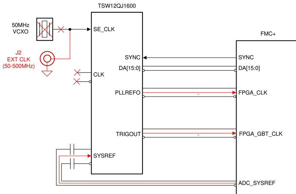
**Figure B-2. Ext Ref to ADC PLL System Block Diagram**
