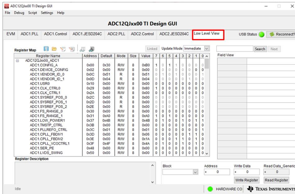
**Figure 4-1. Low-Level Register Control Tab**
