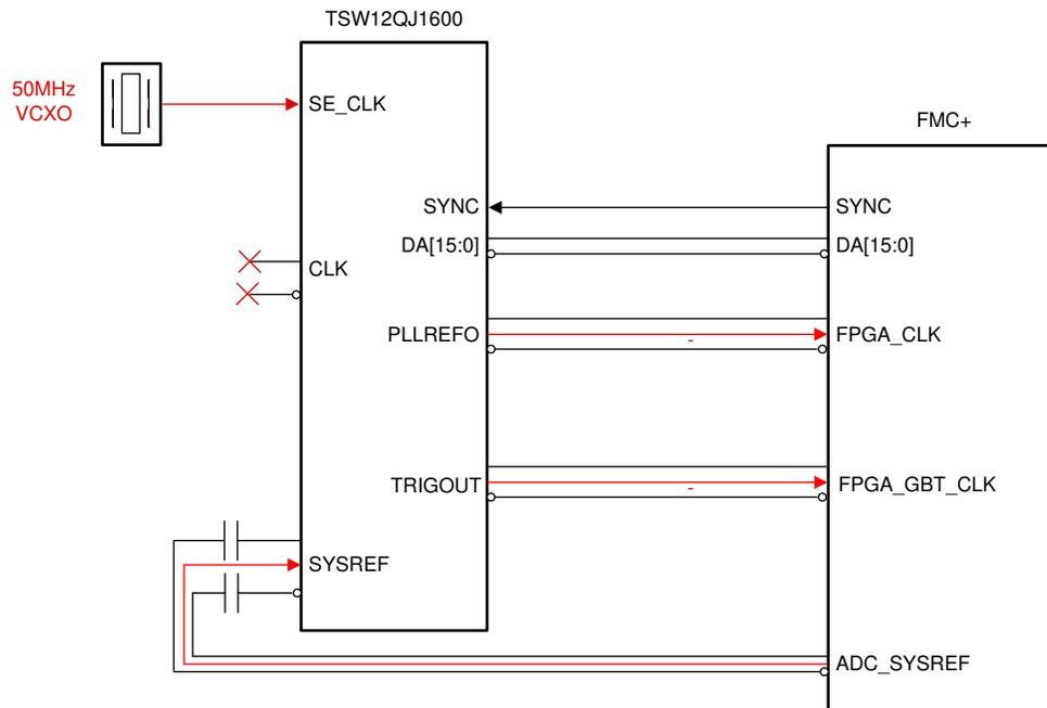
**Figure B-1. Onboard 50M Ref to ADC PLL System Block Diagram**
