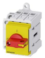
Load disconnector 3LD3, lu 25 A Main switch 3-pole Rated operating capacity at AC-23 A at 400V 9.0kW Installation in distribution boards, Basic switch with selector knob red / yellow with auxiliary switch 10E + 1S
