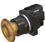
30mm BlackMax, Epoxy Coated Corrosion Resistant Complete Metal Unit Illuminated Push-Pull Operator Full Voltage, 12V AC/DC Incandescent Lamp Mushroom Head Cap Small 1 3/4" (44.5 mm) Plastic, Amber 3 Position Momentary UL Listed, CSA Certified NEMA 1,3,3R,4,4X,12,13 & Automotive Standards
