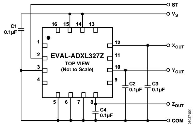
Figure 1. Schematic
