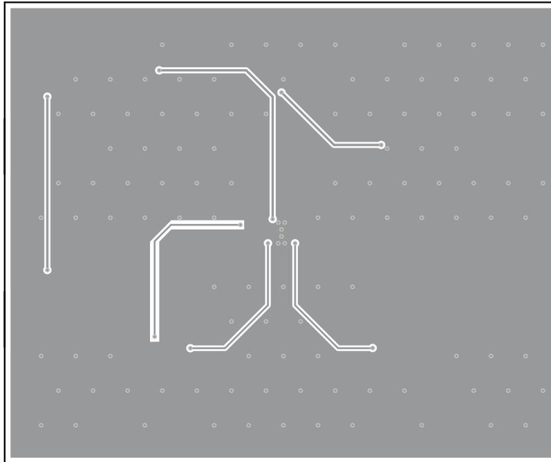
**Figure 4. Bottom Layer Routing**
