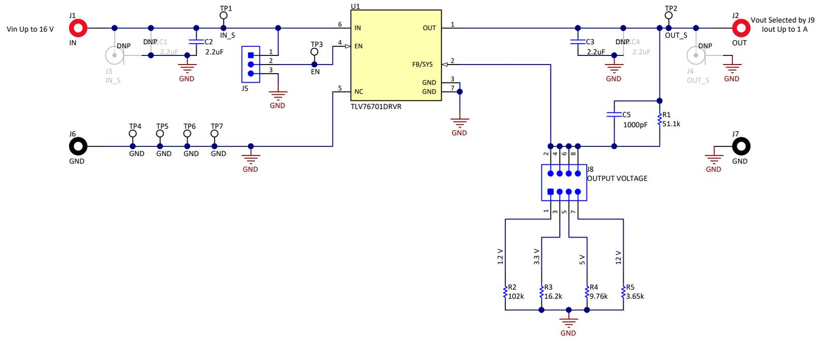
Figure 5. TLV767EVM-014 Schematic
