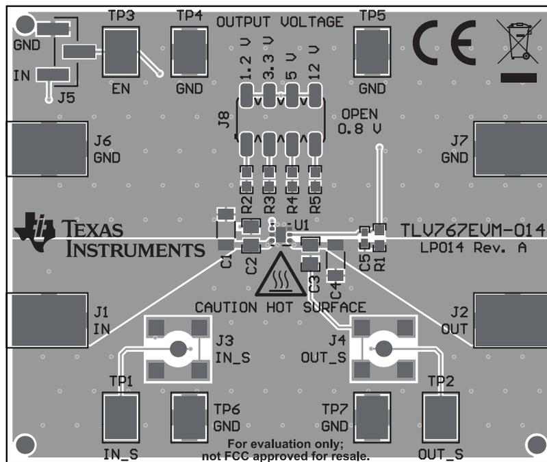
Figure 2. Assembly Layer
