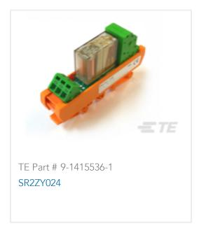
Force-Guided Relay, DC, Monostable, 3A (NO) + 3B (NC), 8 A Contact Rating, 24 VDC Coil Voltage, 250 VAC Contact Voltage, 1.2 W Coil Power, SCHRACK SR6
