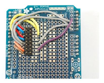
It's not necessary to install all the buttons and lights on the proto shield if you don't want — just the basic header pins are sufficient.
