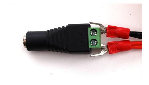
You may receive power cables with different endings, e.g. round instead of spade ends, or maybe with another Molex connector. Just strip the cables and wire directly to the power plug
