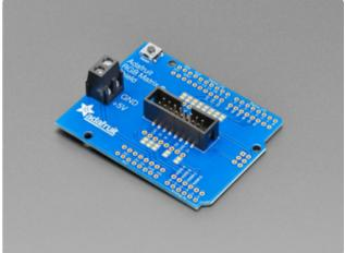
The shield comes with the button, terminal block, and the 16-pin header already soldered on. All you need to do is solder the headers!
