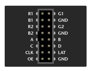
Here's the layout for **32x32** and **64x32** panels. We'll call this "Variant A." Some panels use different labels, but the functions are identical.
