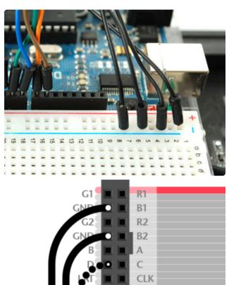
**32x32** and **64x32** matrices require **three** ground connections. **32x16** matrices have **four**.
