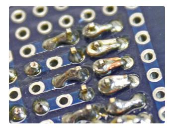
Depending on the make and model of proto shield, some pins are designed to connect in short rows. Others don't. For the latter, strip a little extra insulation and bend the wire to wrap around the leg of the socket from behind, then solder.
