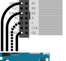
Current Arduino Uno form-factor boards have three ground pins (the third is next to pin 13). If you need additional ground connections — for a 32x16 matrix, or if using an older Arduino board with only 2 ground pins — a solderless breadboard is handy for linking all these pins.
