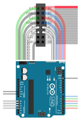
Pins A, B, C and D select which two rows of the display are currently lit. (32x16 matrices don't have a "D" pin — it's connected to ground instead.)
