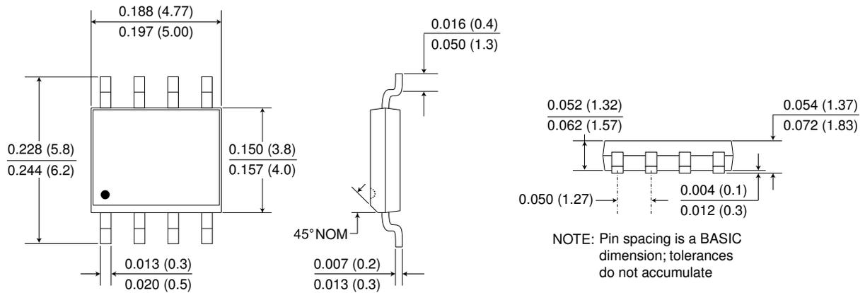
NOTE: Pin spacing is a BASIC dimension; tolerances do not accumulate
