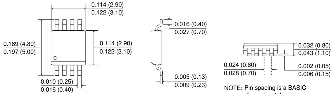
NOTE: Pin spacing is a BASIC dimension; tolerances do not accumulate
