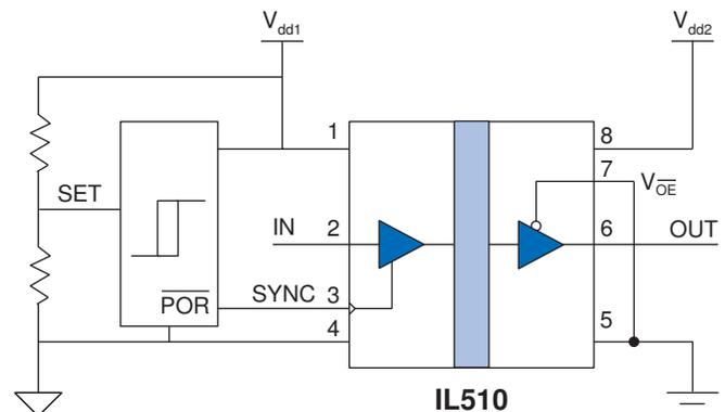
Fig. 1. Typical Power On Reset Circuit for IL510
