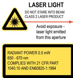
Low-power lasers are, by definition, incapable of causing eye injury within the duration of a blink (aversion response) of 0.25 seconds. They also must emit only visible wavelengths (400 to 700 nm). Therefore, an ocular hazard may exist only if individuals overcome their natural aversion to bright light and stare directly into the laser beam.
