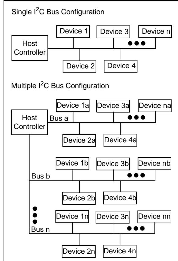
**FIGURE 8-5:** Typical Application I<sup>2</sup>C Bus Configurations.
