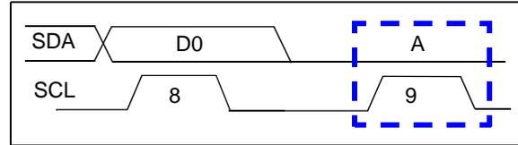
**FIGURE 6-4:** Acknowledge Waveform.
