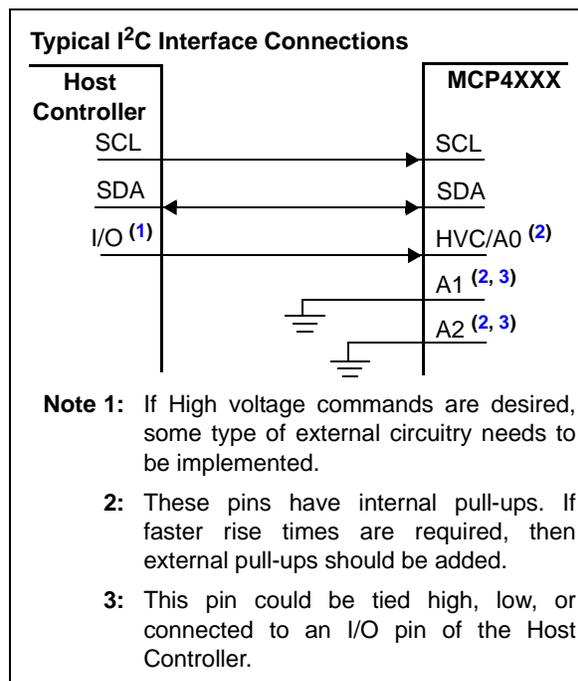
**FIGURE 6-1:** Typical I<sup>2</sup>C Interface Block Diagram.
