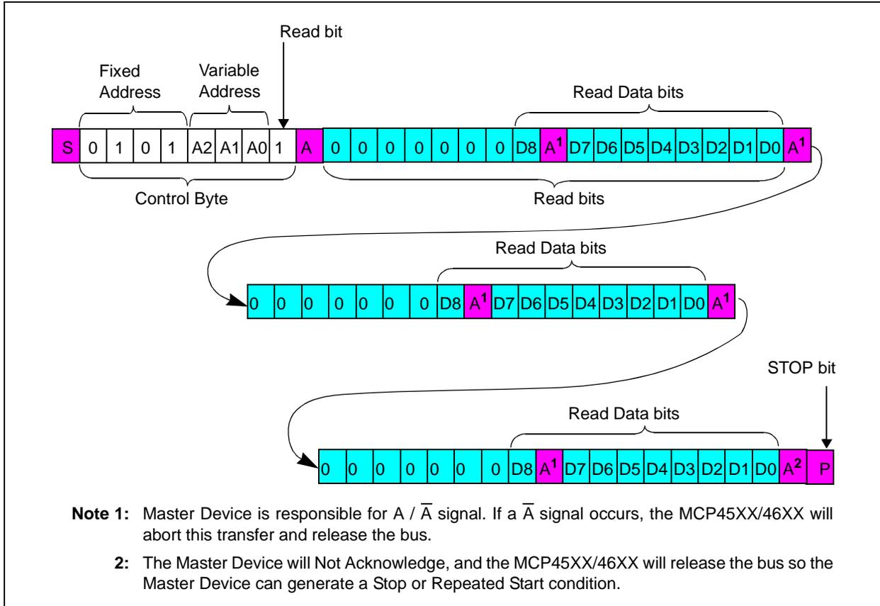
**FIGURE 7-6:** I<sup>2</sup>C Continuous Reads.
