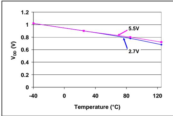
**FIGURE 2-64:** POR/BOR Trip point vs.  $V_{DD}$  and Temperature.
