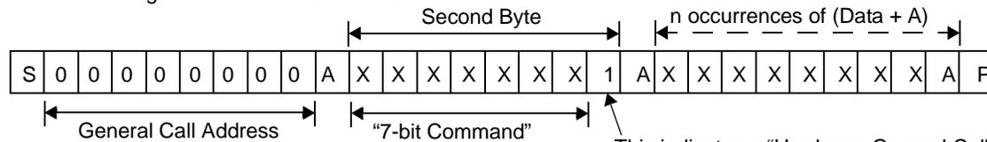
This indicates a "Hardware General Call" MCP45XX/MCP46XX will ignore this byte and all following bytes (and A), until a Stop bit (P) is encountered.
