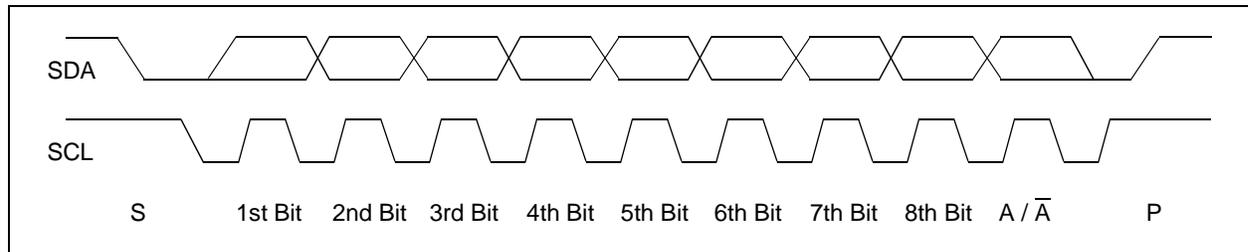
**FIGURE 6-7:** Typical 8-Bit I<sup>2</sup>C Waveform Format.
