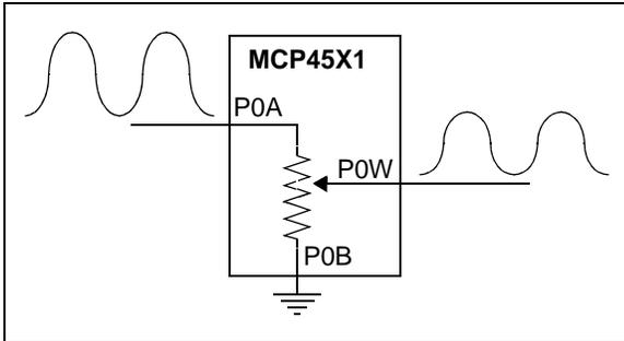
**FIGURE 8-7:** Signal Attenuation Block Diagram - Ground Referenced.
