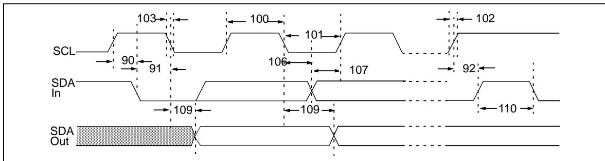
**FIGURE 1-2: I<sup>2</sup>C Bus Data Timing.**
