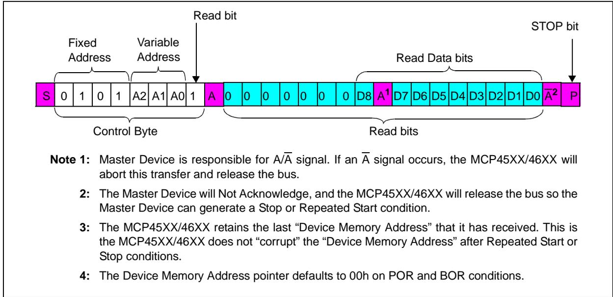
**FIGURE 7-4:** I<sup>2</sup>C Read (Last Memory Address Accessed).
