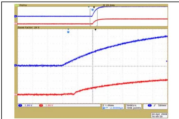
**FIGURE 2-29:**  $10\text{ k}\Omega$  – Power-Up Wiper Response Time ( $1\ \mu\text{s}/\text{Div}$ ).
