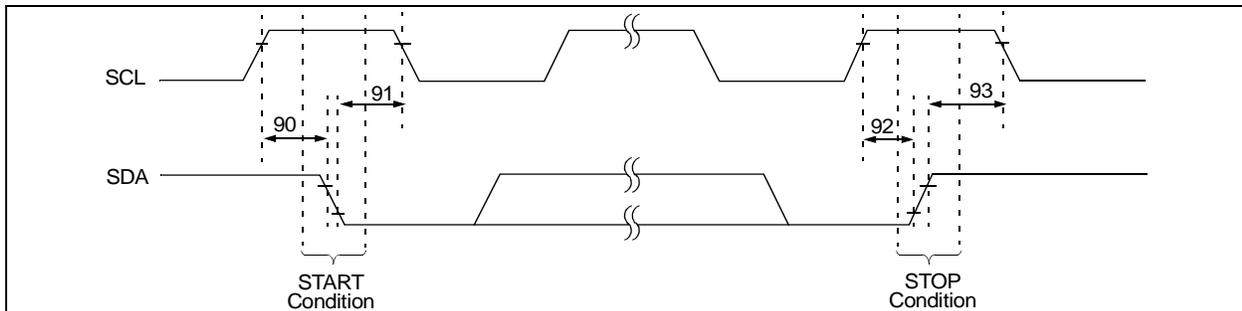
**FIGURE 1-1:**  $I^2C$  Bus Start/Stop Bits Timing Waveforms.
