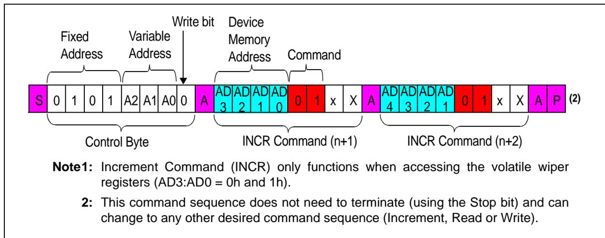
FIGURE 7-7: I<sup>2</sup>C Increment Command Sequence.
