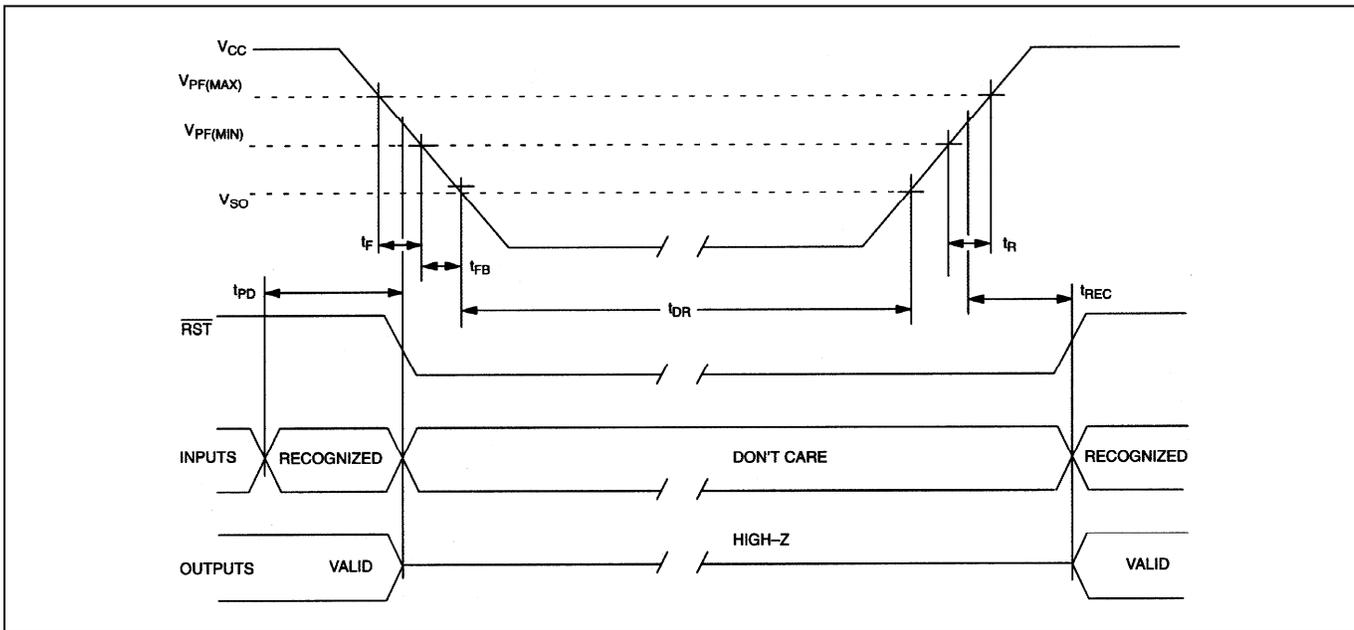
**POWER-UP/DOWN CHARACTERISTICS**(V<sub>CC</sub> = 3.3V ±10%, T<sub>A</sub> = Over the operating range.)
