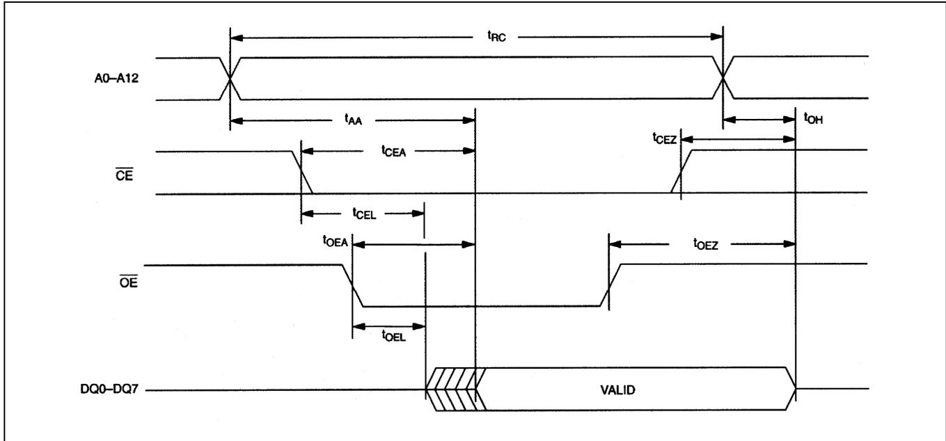
**READ CYCLE, AC CHARACTERISTICS**(V<sub>CC</sub> = 5.0V ±10%, T<sub>A</sub> = Over the operating range.)
