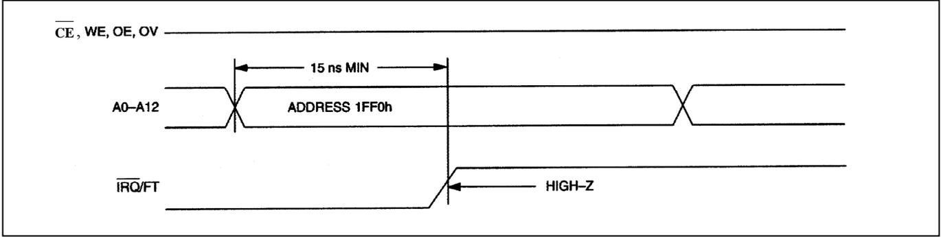
**Figure 3. Clearing  $\overline{\text{IRQ}}$  Waveforms**
