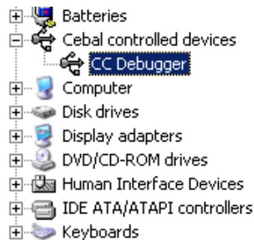
**Figure 1. Verify Correct Driver Installation**
