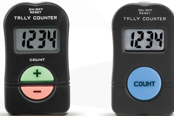
The 18 Series electronic hand tally counter are available with a choice of Add only or Add/Subtract models. Counts are input using large positive action buttons. The Add model has a single count button and the Add/Subtract model has two separate count buttons. The counter is manufactured from impact-resistant plastic, combining lightweight with outstanding durability.
