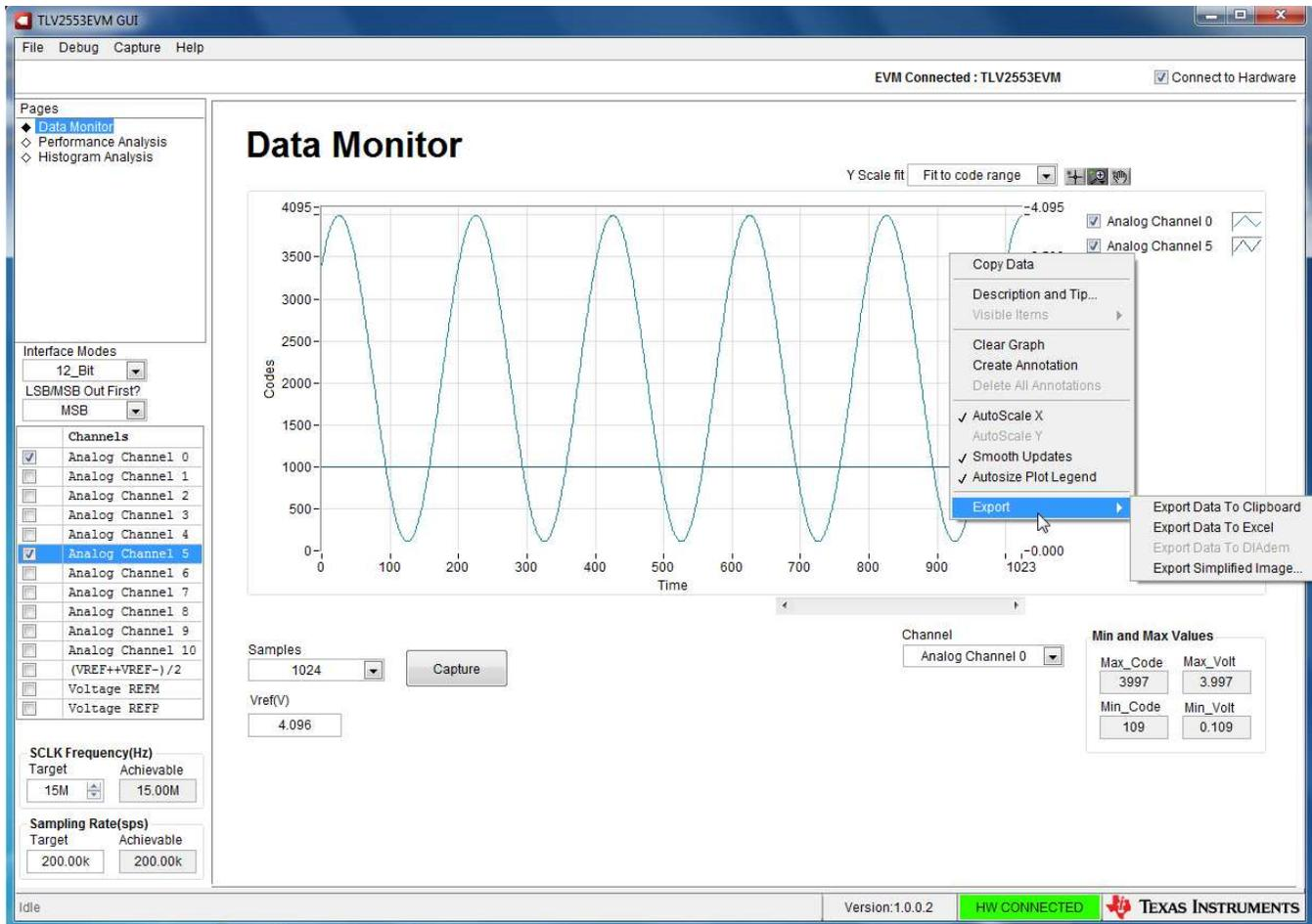
Figure 11. Multichannel Acquisition and Data Export Options
