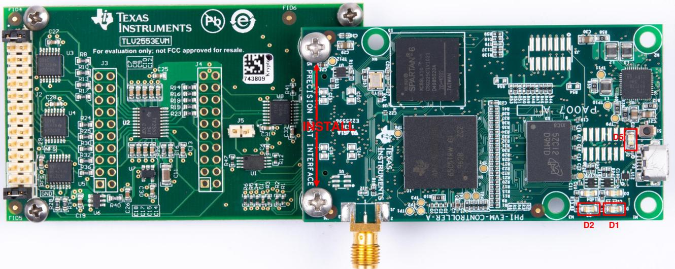
**Figure 8. EVM-PDK Hardware Setup and LED Indicators**
