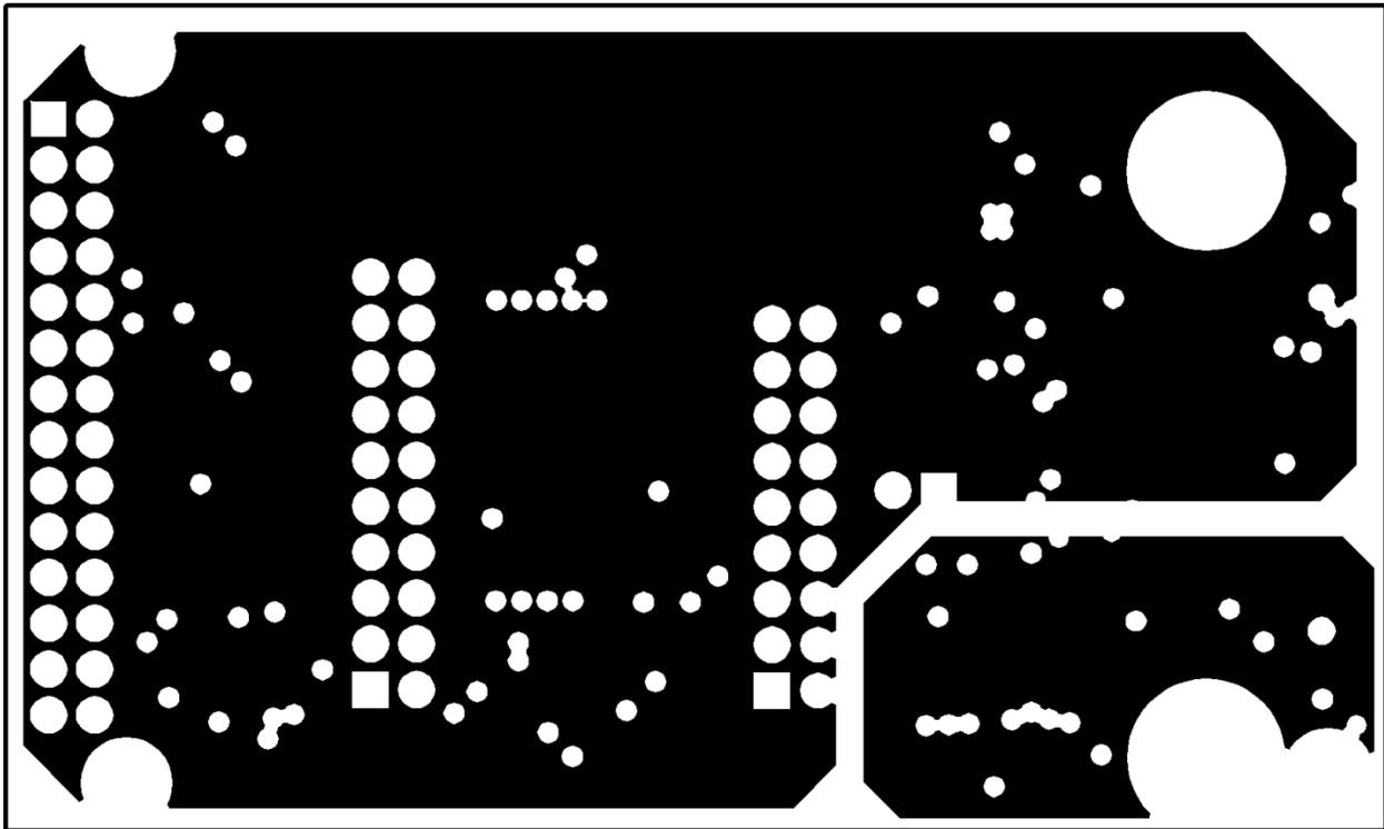
Figure 16. TLV2553EVM PCB Layer 3: Power Planes
