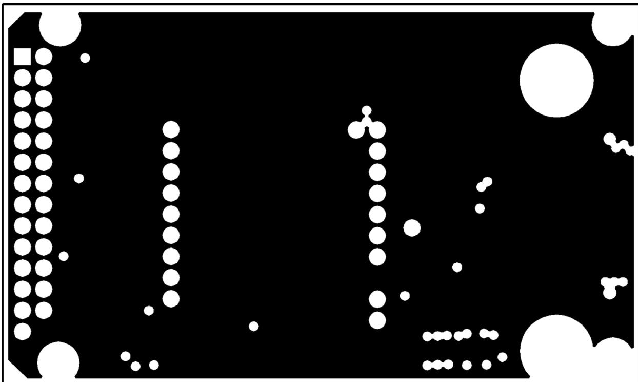
Figure 15. TLV2553EVM PCB Layer 2: GND Plane
