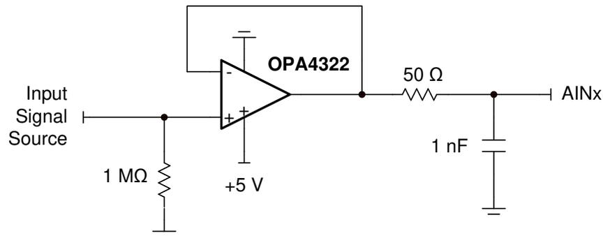
**Figure 1. Input Signal Path Schematic (Single Channel)**
