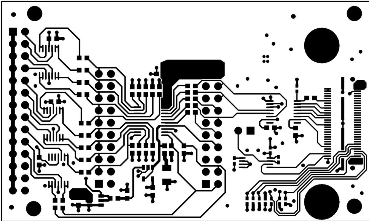
Figure 14. TLV2553EVM PCB Layer 1: Top Layer
