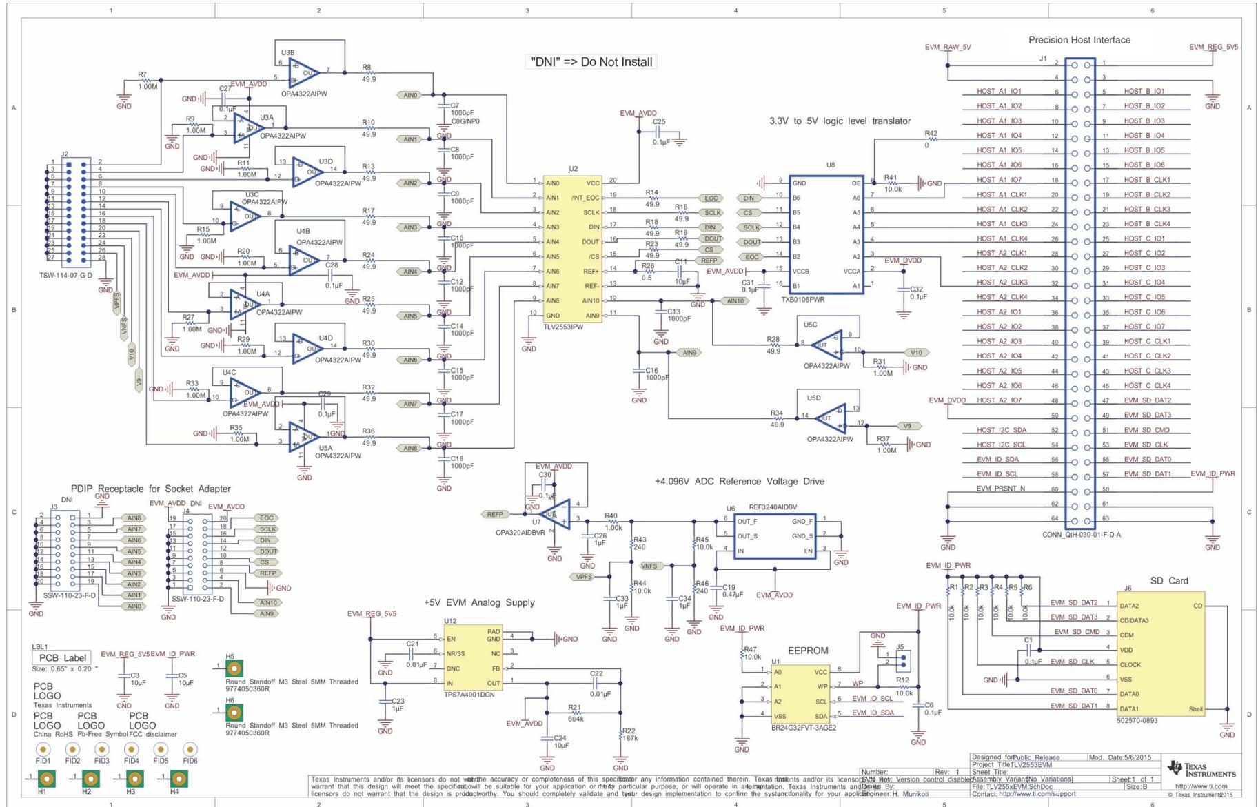
Figure 18. Schematic Diagram of the TLV2553EVM PCB
