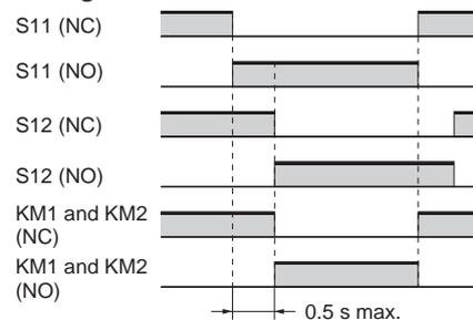
Input time difference operates only when the difference is 0.5 s max.
