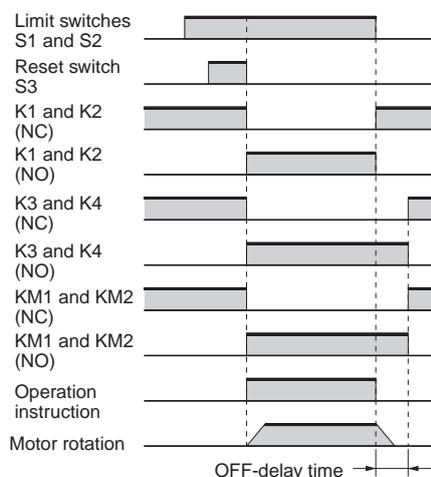
**G9SA-321-T□ (24 VAC/VDC) + G9SA-EX031-T□ with 2-channel Limit Switch Input/Manual Reset**
