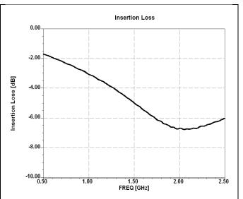
In order for Xinger surface mount delay lines to work optimally, there must be  $50\Omega$  transmission lines leading to and from all of the RF ports. Also, there must be a very good ground plane under the part with a number of plated thru holes to ensure proper electrical performance. If any of these conditions are not satisfied, insertion loss, average delay and VSWR may not meet published specifications.
