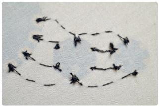
Stitching the sensor into a project is easy-just line up the sensor so its adjacent to the SDA/SCL pins on Flora or another I2C sensor, and stitch the four connections with conductive thread. This is covered in more detail in the Flora
