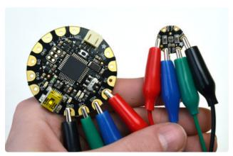
To test the sensor before sewing it into a project, use alligator clips to hook up the 3.3v, SDA, SCL, and GND pins.
