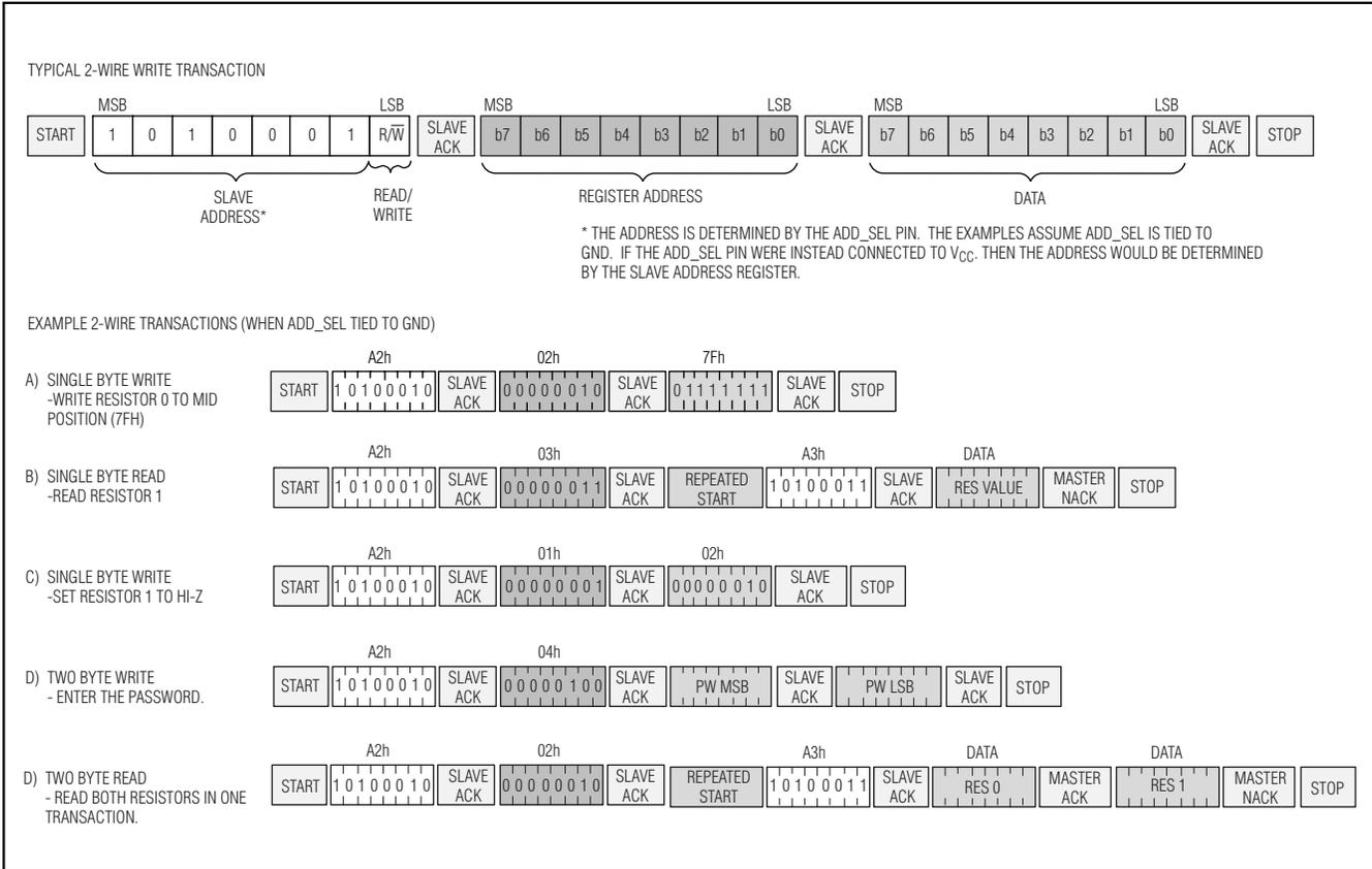
Figure 2. I<sup>2</sup>C Communication Examples
