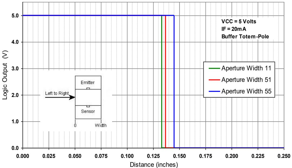
Logic Output vs Top to Bottom Bocking Distance (Y-Axis Blocked)
