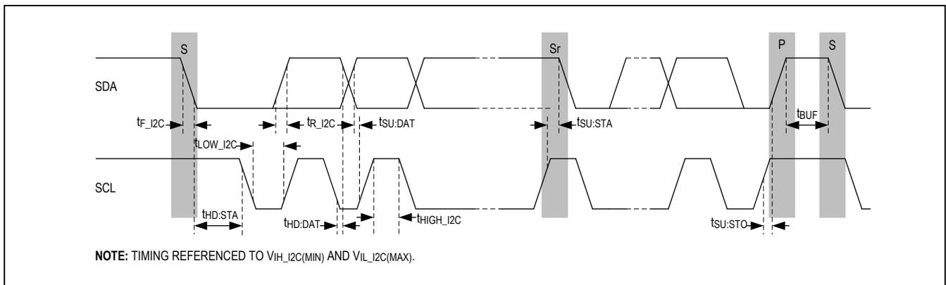
Figure 7. I<sup>2</sup>C Bus Controller Timing Diagram
