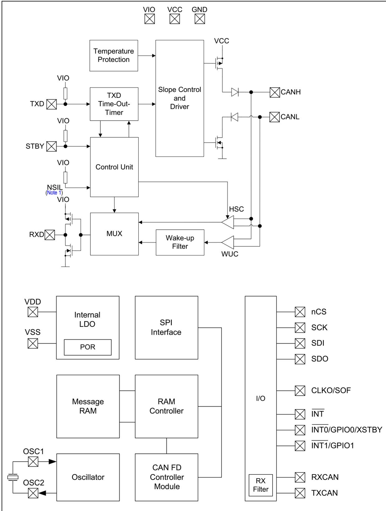
**Note 1:** NSIL is not an externally available signal on this device and instead is pulled to VIO.
