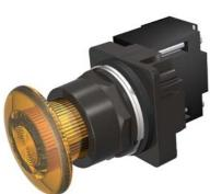
30mm BlackMax, Epoxy Coated Corrosion Resistant Complete Metal Unit Illuminated Push-Pull Operator Full Voltage, 6V AC/DC Incandescent Lamp Mushroom Head Cap Small 1 3/4" (44.5 mm) Plastic, Amber 3 Position Pull-Momentary/Push-Maintained UL Listed, CSA Certified NEMA 1,3,3R,4,4X,12,13 & Automotive Standards
