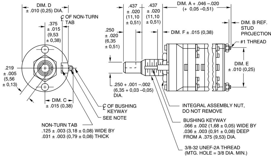
**Note:** Common location for a single pole per deck switch. For common location on multi-pole switches, see circuit diagrams.
