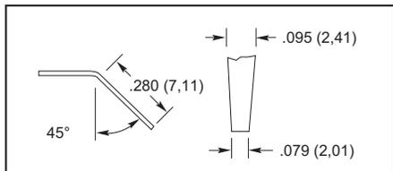
Used in place of conventional solder lug terminals. Taper tab terminals are gold plated.
