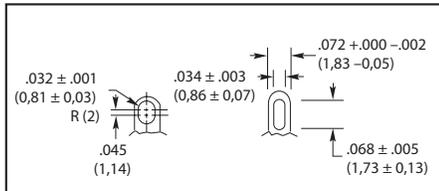
Series 08A, 09A, 42H, 42M, 44H, and 44M: Lug terminals for several wires; standard in Series 08M, 09M, 53, 57, and 59 switches.
