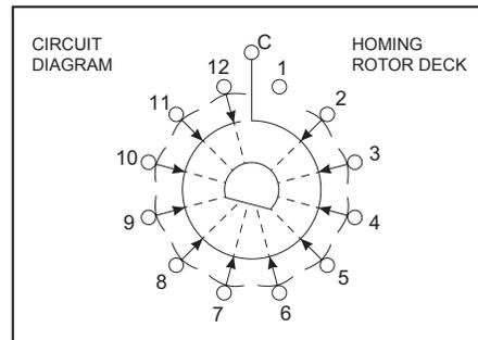
connected to the common, and terminal 1 is open. In position 2, terminal 3 thru 12 and 1 are connected to the common, and terminal 2 is open. A homing rotor deck will function for 25,000 mechanical cycles of operation.
