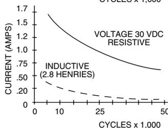
**Voltage and Load:** As listed in the chart One cycle is 360° rotation and a return through all switch positions to the starting position. The data for the curves was measured at sea level, 25°C and 68% relative humidity.
