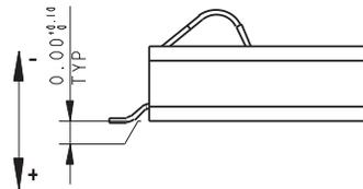
CONTACT TAILS TO BE WITHIN A 0.1 COPLANARITY RANGE WHEN INSULATOR IS SITTING ON DATUM FACE.
