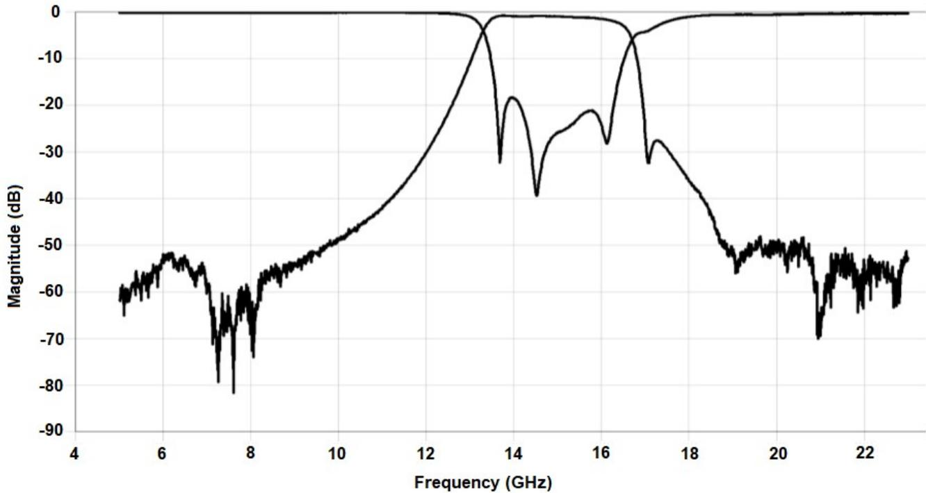
\*Typical de-embedded measured performance mounted on a connectorized test fixture. DEB is 0.010in RO4350B with 50.0Ohm CPW ground traces going into the ports at room temperature.
