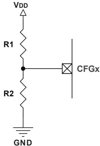
Note: It is recommended that R1 and R2 be greater than 100 k $\Omega$  for lower power consumption.
