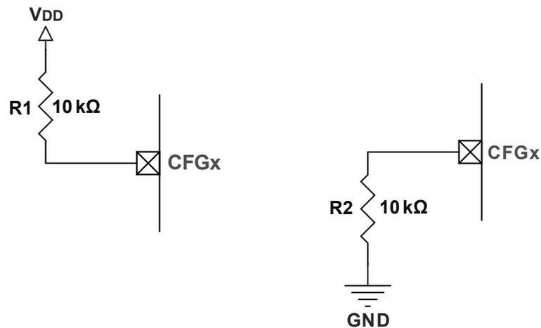
The pull-up/pull-down resistor is a pre-cautionary recommendation, as MTCH1060 will pull the CFGx neither to the V<sub>DD</sub> nor to the GND during the operation.
