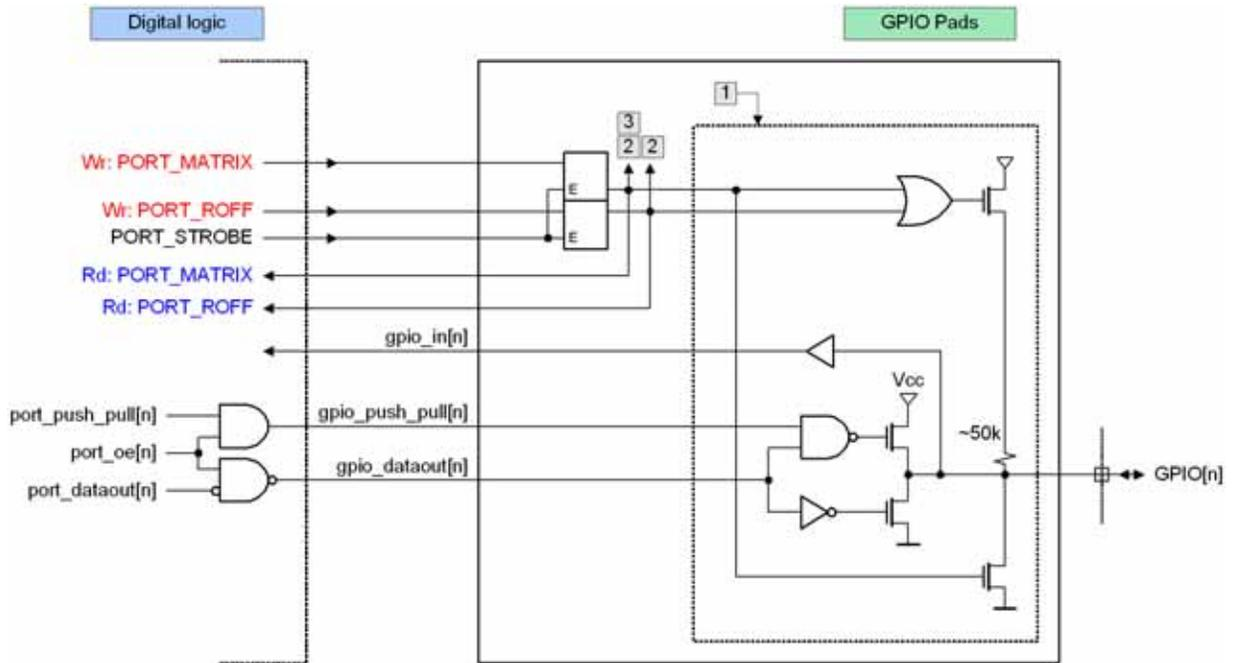
**Figure 30.2. GPIO[3:1] Functional Diagram**
