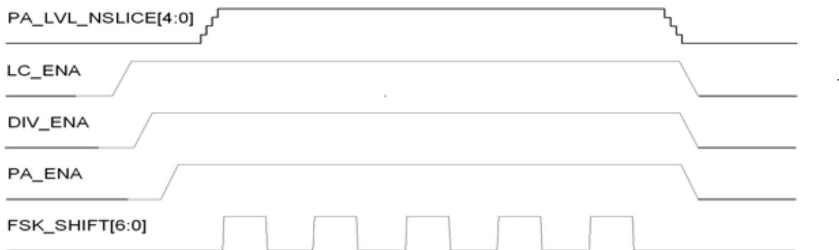
Figure 13.2. FSK Timing Example
