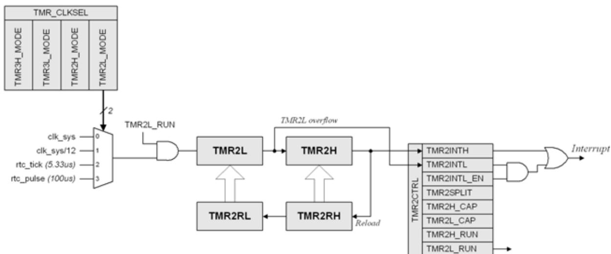
Figure 34.2. Timer 16-bit Mode Block Diagram (Wide Mode)
