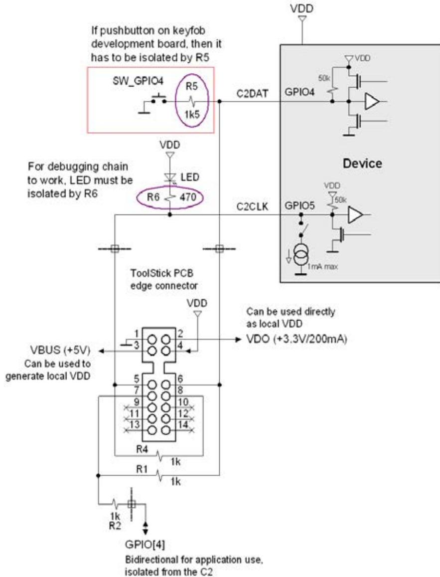
**Figure 35.2. 14-Pin C2 ToolStick Connection to Device**
