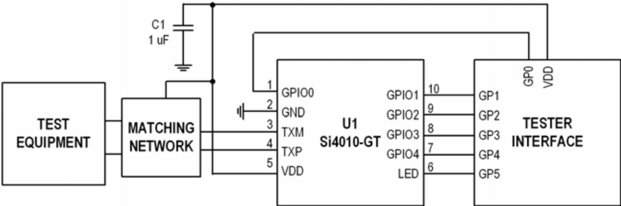
Figure 2.1. Test Block Diagram with 10-Pin MSOP
