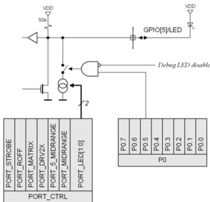
Figure 30.5. GPIO[5] LED Driver Block Diagram
