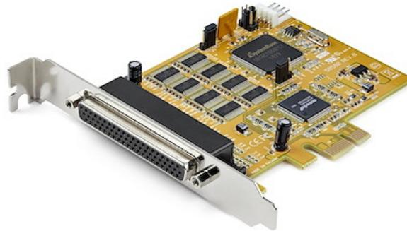
Add eight RS-232 DB9 serial ports to your desktop computer, through a PCIe expansion card slots. This PCI express serial card, with 8-port breakout cable, provides you with multiple ports to connect a wide variety of serial peripherals, at speeds of up to 921.4Kbps.
