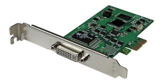
This all-in-one PCI Express capture card lets you record 1080p HD video and stereo audio to your computer system. With multiple video inputs including HDMI, DVI, VGA and component, the capture card can record original content from various sources such as computers, camcorders, security systems, POS terminals, and servers. With H.264 encoding, this is the perfect solution for capturing high-definition video for editing, compiling, and archiving.
