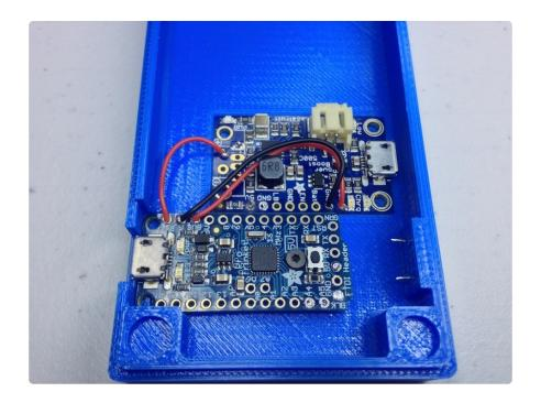
Use three short wires to connect the power lines between the PowerBoost and the Pro Trinket.
