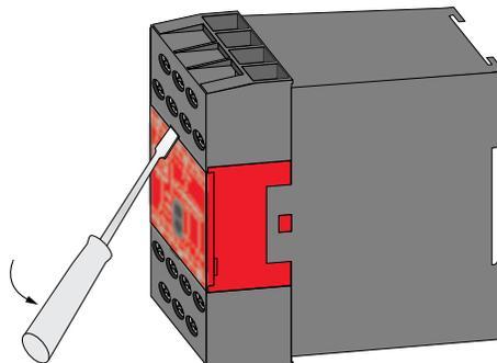
Figure 7. Removal of Terminal Blocks
