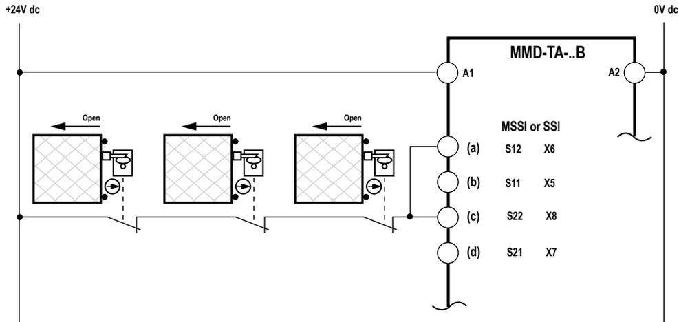
Figure 26. MSSI or SSI Category 2 interfacing: positive opening
