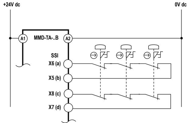
Figure 25. SSI Category 4 interfacing: positive-opening E-stop switch(es)
