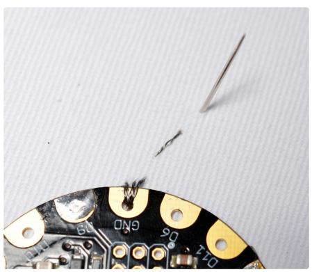
The thread must travel between components to connect them, while avoiding other paths of conductive thread in the circuit. The thread acts like uninsulated wire or traces on a circuit board, but this circuit board is made out of fabric!
