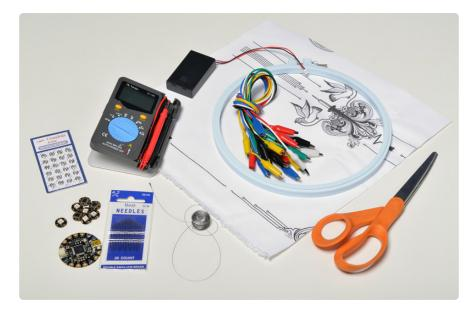
You'll need some conductive thread, scissors, needles, fabric or a garment, a battery pack, and the following:
