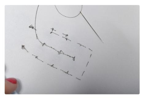
Keep power and ground lines far apart from each other. A short between power and ground will prevent your project from working and may even cause your battery to heat up.
