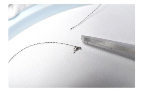
When dry, trim the tail end of the thread very closely to the sealed knot. Now you can continue stitching with the long tail to connect up different parts of your circuit!
