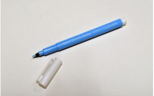
Use a water-disolvable marker to plan out your circuit traces.
