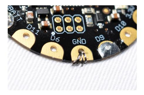
Repeat with a few more stitches to make a secure mechanical and electrical connection.
