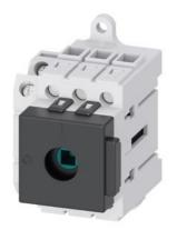
Load disconnector 3LD3, lu 16 A Main switch 3-pole Rated operating capacity at AC-23 A at 400V 7.5kW Installation in distribution boards, Basic switch without Knob-operated mechanism with auxiliary switch 1OE + 1S
