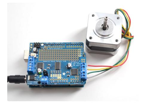
You must also supply 5-12VDC to power the motor. There are two ways to do this
