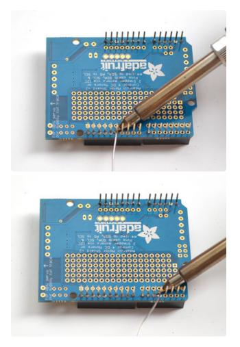
Once you've tacked and straightened all the headers, go back and solder the remaining pins for each header.
