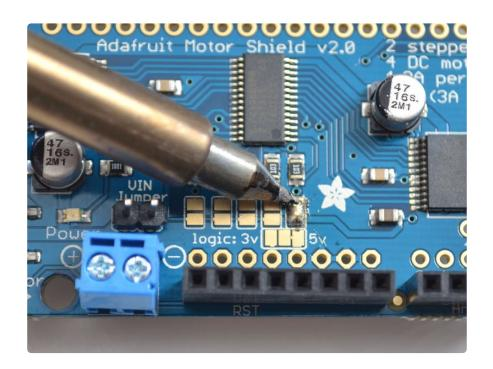
Board 0: Address = 0x60 Offset = binary 0000 (no jumpers required) Board 1: Address = 0x61 Offset = binary 0001 (bridge A0 as in the photo above) Board 2: Address = 0x62 Offset = binary 0010 (bridge A1, to the left of A0) Board 3: Address = 0x63 Offset = binary 0011 (bridge A0 & A1, two rightmost jumpers) Board 4: Address = 0x64 Offset = binary 0100 (bridge A2, middle jumper)
