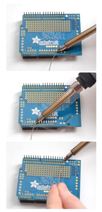
Tack one pin of each header, to get them set in place before more soldering. If the headers go crooked you can re-heat the one pin while re-positioning to straighten them up
