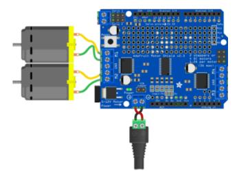
Connect the two motor wires from the first motor to the M1 terminal on the Shield. Connect the two motor wires from the second motor to the M2 terminal on the Shield.
