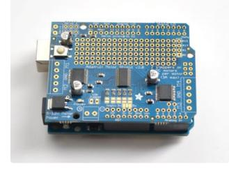
Place the assembled shield on top of the header-ed Arduino so that all of the short parts of the header are sticking through the outer set of pads
