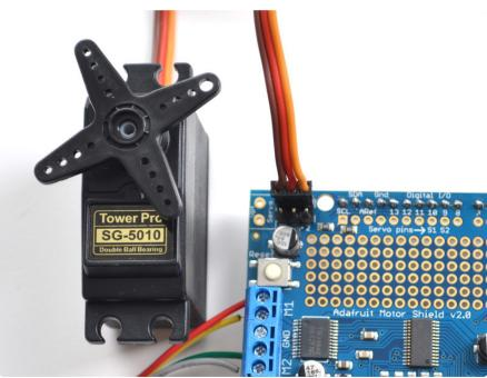
Hobby servos are the easiest way to get going with motor control. They have a 3-pin 0.1" female header connection with +5V, ground and signal inputs. The motor shield simply brings out the PWM output lines from Arduino pins 9 and 10 to two 3-pin
