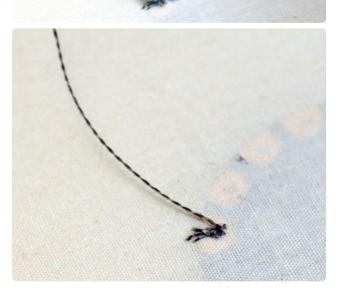
Dab a little Fray Check or clear nail polish on the knot while holding it tight. This will prevent the knot from coming undone and creating unwanted shorts in your circuit. Trim the tail very close to the knot.
