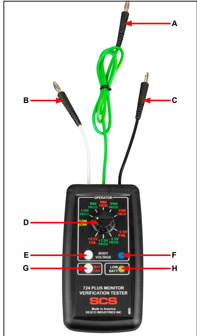
Figure 2. 724 Plus Monitor Verification Tester features and components
