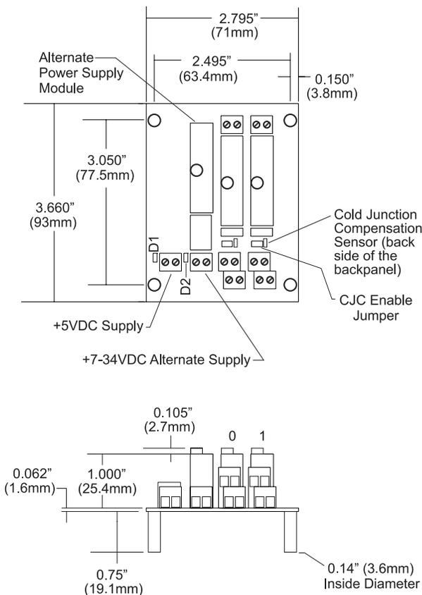
Figure 1: 8BP02 Analog I/O Backpanel
