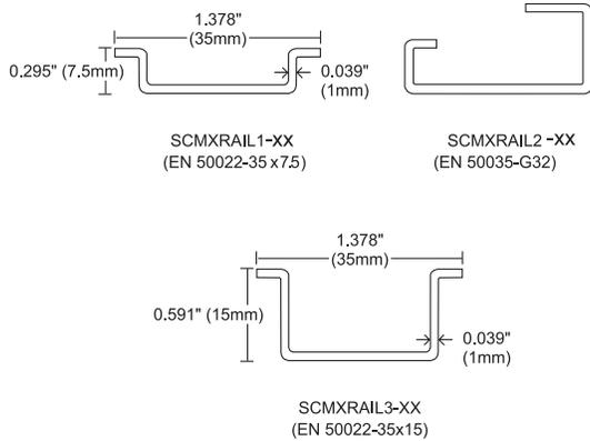
Figure 8: DIN-rail Styles
