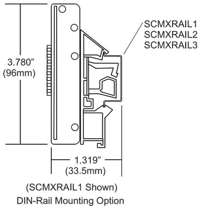
Figure 9: 8BPxx-2, 8BPxx-3 Backpanel DIN-rail Mounting Option
