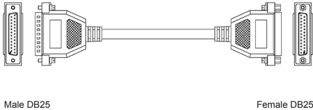
Figure 5: SCMXCA006-XX System Interface Cable
