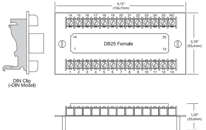
Figure 6: 8BXIF Universal Interface Board Dimensions
