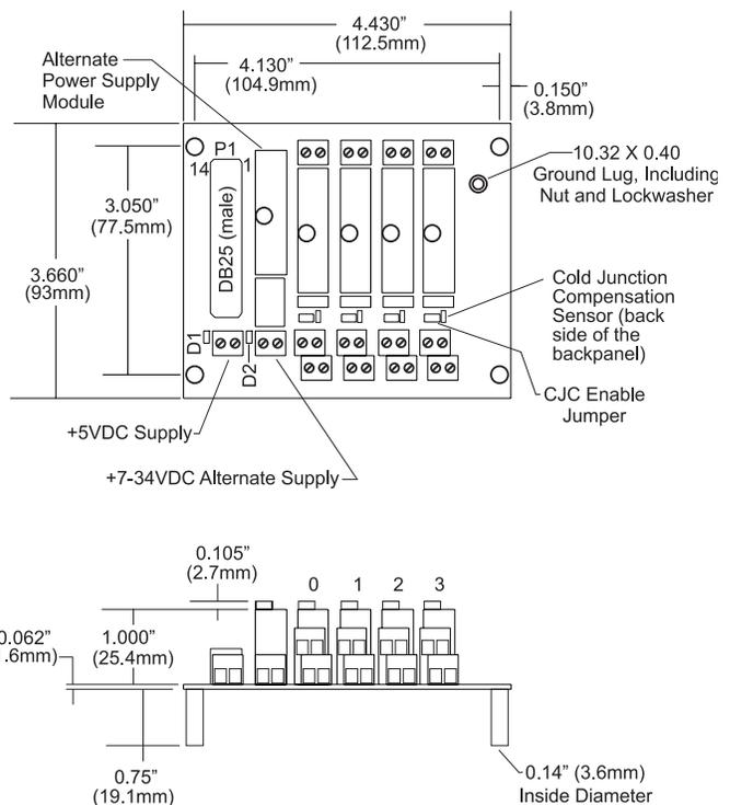
Figure 2: 8BP04 Analog I/O Backpanel
