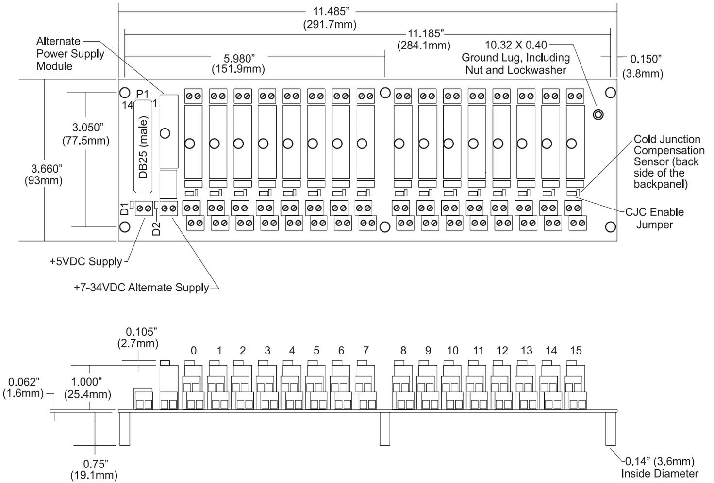
**Figure 4: 8BP16 Analog I/O Backpanel**
