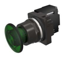
30mm BlackMax, Epoxy Coated Corrosion Resistant Complete Metal Unit Illuminated Push-Pull Operator Full Voltage, 120V AC/DC Incandescent Lamp Mushroom Head Cap Small 1 3/4" (44.5 mm) Plastic, Green 3 Position Pull-Momentary/Push-Maintained UL Listed, CSA Certified NEMA 1,3,3R,4,4X,12,13 & Automotive Standards
