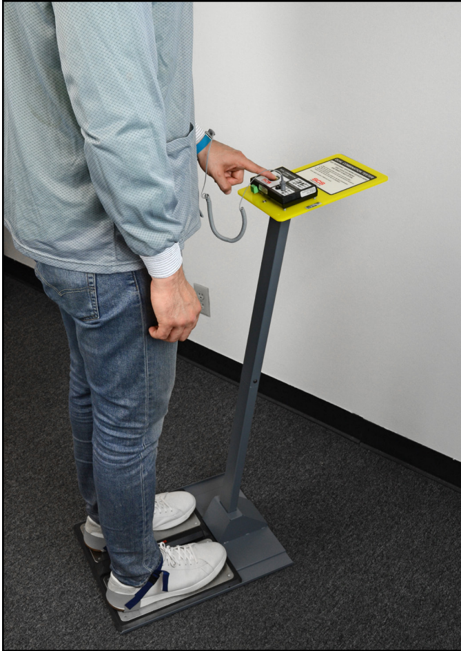
Figure 13. Using the Dual Combination Tester with the 770759 Stand
