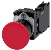
Mushroom pushbutton, 22 mm, round, plastic, red, 40mm, latching, pull-to-unlatch mechanism, with holder, 1 NO+1 NC, spring-type terminal, with laser labeling, upper case
