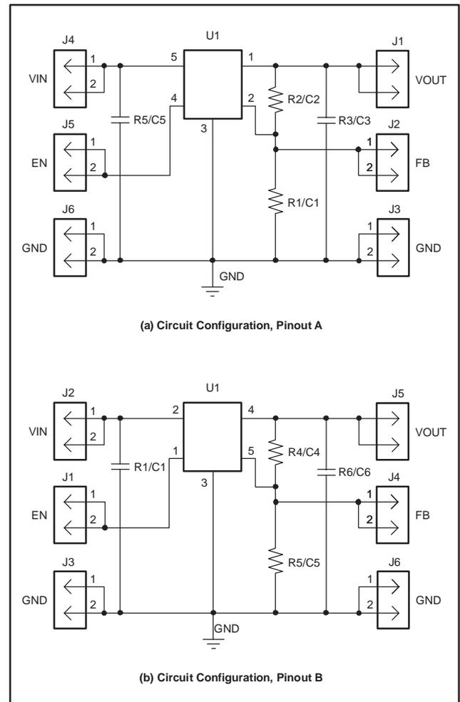
**Figure 2. Example Board Configurations for Evaluating LDOs in the TO220 or TO263 packages.**
